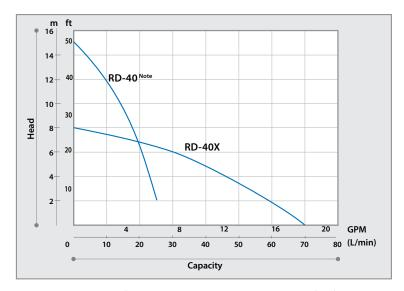
Note: Do not exceed 6.6 GPM in operation, or cavitation may take place. The above curves are based on operation with a 5V external control signal.
