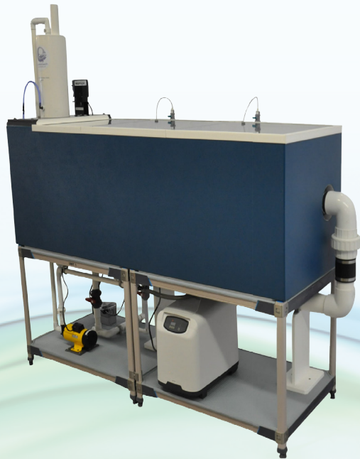
A closed-circuit 424-L (112 gal) tank on a plastic frame
